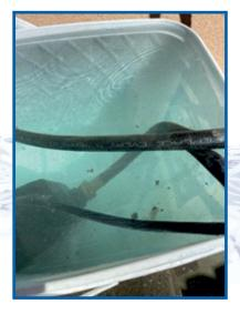
Following flush with water, again virtually **no**scale debris
